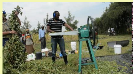
Pic 12: Chopping sweet potato vines with a chaff cutter. (source Mazingira Centre on Innovation Feeding Approaches for Dairy Farmers)
